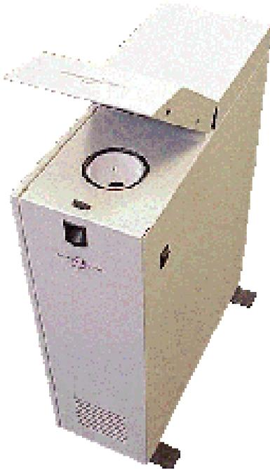
The BrillianceScope measures the diamond in a controlled lighting environment consisting of multiple lighting angles. To initiate the evaluation process, the gem is placed within a three-inch integrated sphere with a one-inch hole in which the diamond is firmly positioned. If you draw a direct line from the 2.5-inch ring light through the one-inch hole directly to where the diamond rests, an angle of light is created.
