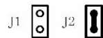
(c) J1 open circuit, J2 short circuit CW/CCW mode and effective at upward-rising edge
