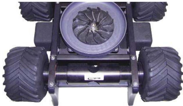
A bottom view of the ROV showing the Pittman brushed dc motors and the planetary gearheads. The LBC offers a powerful size/weight ratio (21 in. x 19.7 in. x 15.7 in.) and the entire assembly weighs 61.7 lb.
