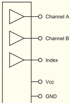
**Figure 5:** Connector pin-out for a three-channel encoder with single ended outputs.
