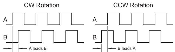
Figure 2: Encoder waveforms indicating a change in direction.
