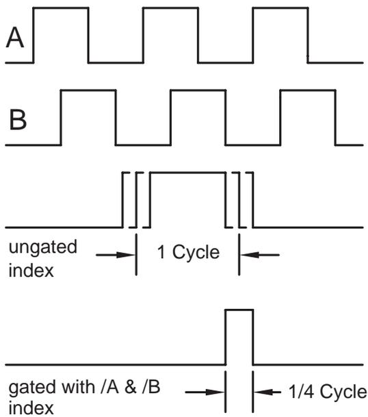
**Figure 4:** Three-channel incremental encoder waveform with a comparison of ungated and gated forms of index signals.
