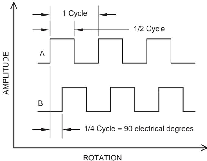
Figure 1: Two-channel incremental encoder waveform.
