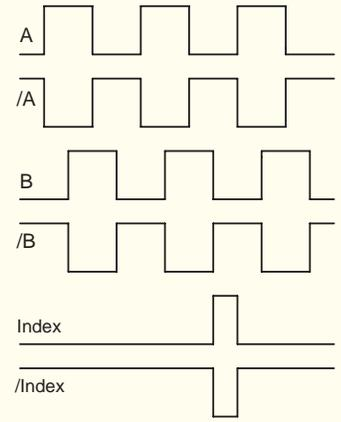
**Figure 6:** Differential line driver encoder waveform.
