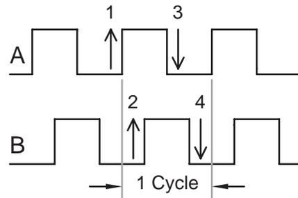
Figure 3: Quadrature counting of encoder signals.
