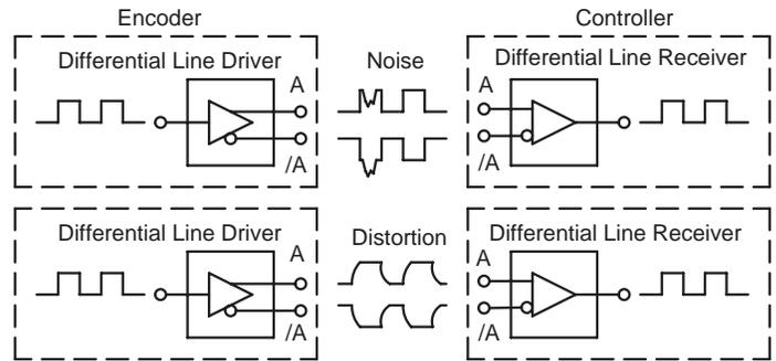
**Figure 7:** Differential line driver signal conditioning.
